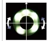
The camera's automatic horizontal adjustment function allows it to turn according to its orientation inside of the pipe. As it always keeps the video image facing upwards, the operator can easily judge the situation inside the pipe. The positioning of the LEDs has been improved to point more upwards so as to avoid darker images at the top or further down the pipe.
