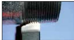
With 20 mm-wide profiling dies, the load is reduced, which makes it easy on the motor.
