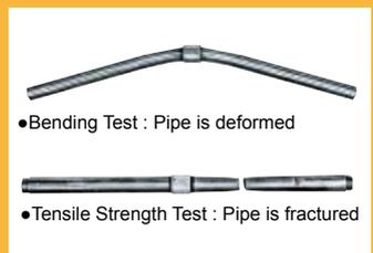
Fig. 5 In strength tests, there was no effect on the thread. The pipe itself became deformed or fractured.
