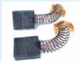
To access and replace the brushes, remove the side and bottom covers with a screwdriver. The brushes can be changed easily, even if they wear out while working at a construction site.
