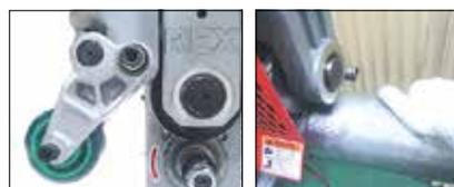
Guide roller prevents the pipe from detaching and eliminates vibration, so there's no need to place your hand on the pipe.
