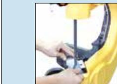
Fig.5 Contour cutting for small steel material
