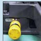
Fig.8 Cutting Load Adjuster (LL, L, M, H)
