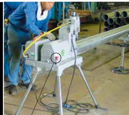
Raise the red knob on the head lock pin to release the self-centering head.
