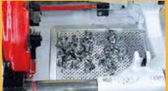
Fig. 2 Chips from roll threads
