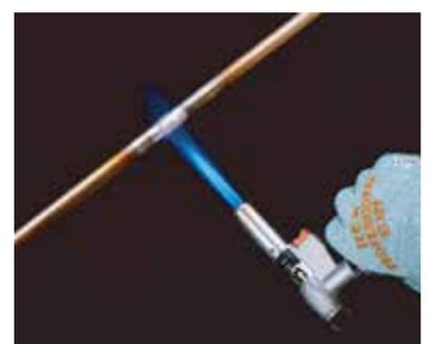
Can be used in inverted position
